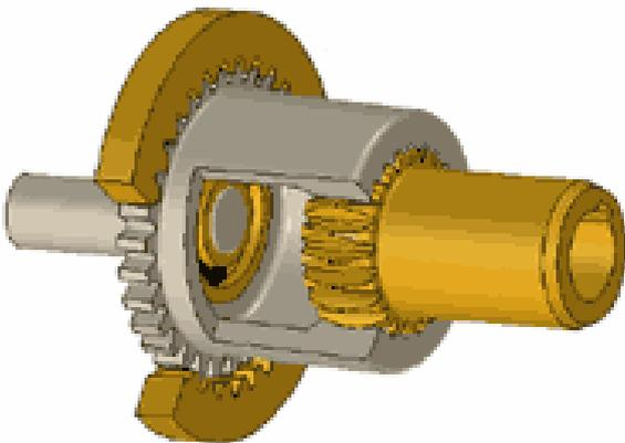
This gear principle is used in applications which require high reduction ratios with perfect accuracy and reliability as in rotary/linear actuators, robotics, high performance electronic instruments and high torque industrial applications. The Oden gear is covered by patents world-wide.
