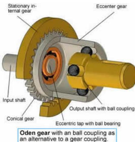
To transmit the slow eccentric rotation of the gear to a centric rotation to the output shaft you may use some kind of coupling. Oden gear has a more simple and reliable solution: The eccenter gear consists of a cylindrical "pipe" with a slightly conical gear placed at one end of it and in the other end an internal coupling. The gear is making a conical movement around the centre point of the coupling. The eccenter on the input shaft has a small balance weight.
