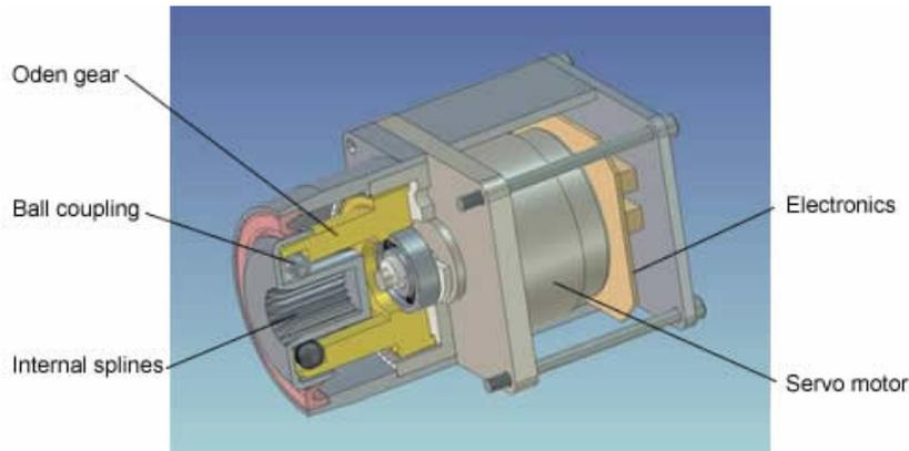
The Oden gear system can also be used as OEM-products. An example to the left, a servo unit using Oden gear. The servo unit is connected to the driven load which have a splined shaft in bearings. This design gives a backlash free servo. The ball coupling in the Oden gear accepts misalignments between the servo unit and the driven shaft.
